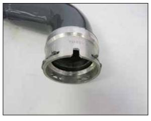
7. Remove the retaining clip and O-ring from the engine side of the factory "Hot Side" charge tube and install them into the "Hot Side" K&N charge tube. NOTE: notice the direction the lip is pointed on the O-ring and be sure to position the same direction in the K&N coupler.
