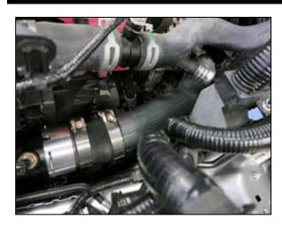
14. Install the K&N "Cold Side" charge tube into the coupler, then position the tube onto the engine inlet and push the tube onto the inlet until an audible "click" is heard as the retaining clip locks onto the inlet. Position the tube and coupler for best fit and then secure the hose clamps. Position the "Cold Side" charge tube for best fit and then secure the hose clamps.
