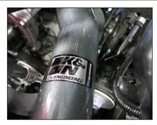
15. Apply the K&N decal to the "Cold Side" charge
