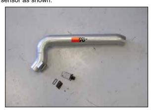
10. On vehicles equipped with a humidity sensor, install the sensor into the K&N® intake tube and secure with the provided hardware. On vehicles that are not equipped with a humidity sensor, install the provided gasket onto the block off and then install the block off into the K&N® intake tube and secure with the provided hardware.
