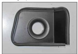
25. Install the provided edge trim onto the heat shield as shown.
