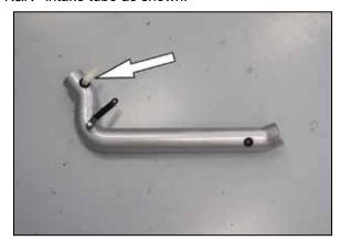
13. Install the  $90^{\circ}$  vent fitting into the grommet installed into the K&N® intake tube as shown.
