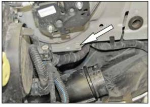
21. Remove the inner fender bolt shown.
