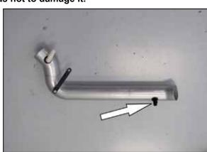
15. Remove the O-Ring from the sensor and then install the sensor into the grommet installed into the  $K\&N^{\otimes}$  intake tube.
