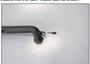
14. Remove the inlet air temperature sensor from the factory air filter housing.
