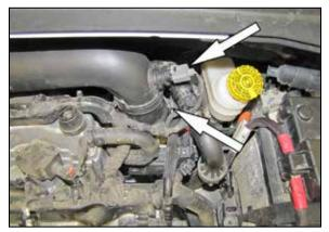
3. Disconnect the inlet air temperature sensor electrical connection, unhook the heater hose from the clip securing it to the intake tube and then loosen the hose clamp that secures the intake tube to the throttle body.
