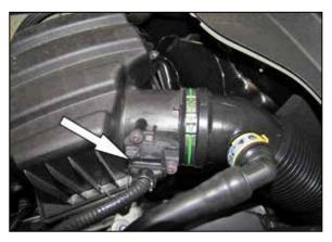
5. On vehicles equipped with a humidity sensor, Disconnect the wiring harness from the sensor.
