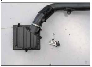
9. On vehicles equipped with a humidity sensor, remove the two screws securing the sensor into the factory air filter housing and then remove the sensor as shown.
