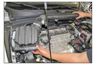
7. Dislodge the air filter housing from the mounting grommets and then remove the complete intake system from the vehicle.
