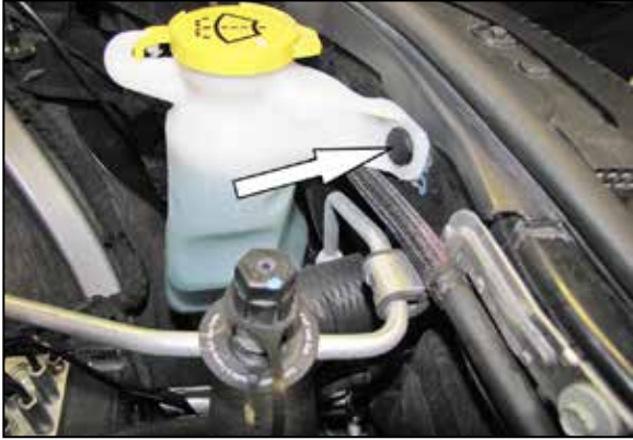
8. Remove the retaining clip that secures the windshield washer bottle to the core support. NOTE: The retaining clip will be reused in a later step.
