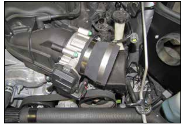
17. Install the step coupler (08497) onto the throttle body and secure with the provided hose clamp.
