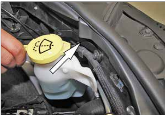
10. Install the provided heat shield mounting bracket onto the core support and secure with the factory bolt from the previous step.
