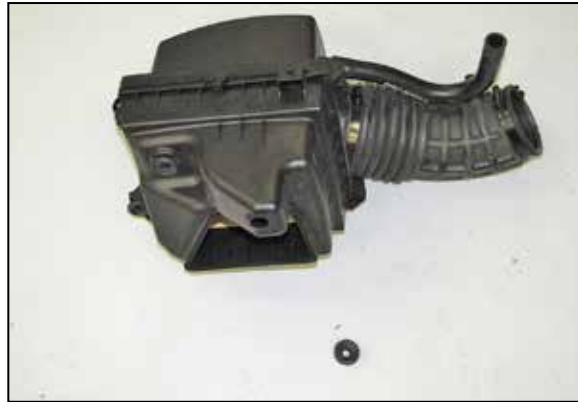
14. Remove one of the factory mounting grommets from the air filter housing assembly as shown.
