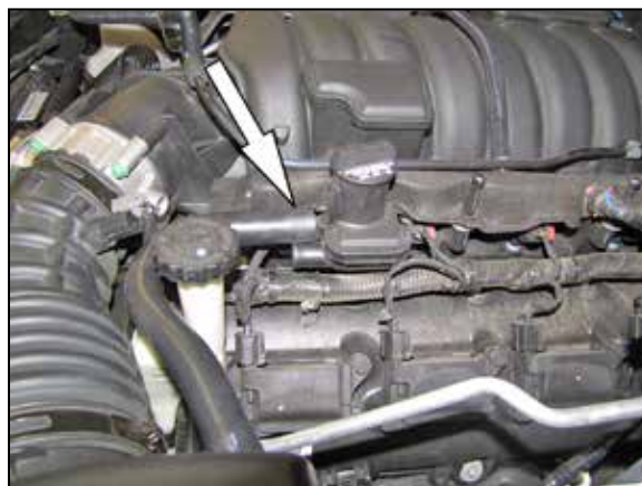
4. Disconnect the crank case vent hose from the valve cover port.
