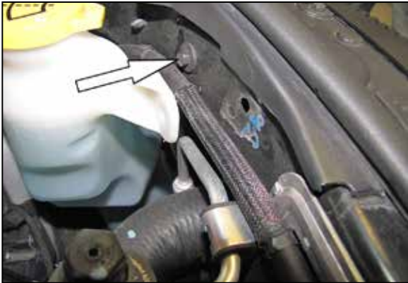
9. Remove the core support bolt shown. NOTE: This bolt will be reused in the next step.
