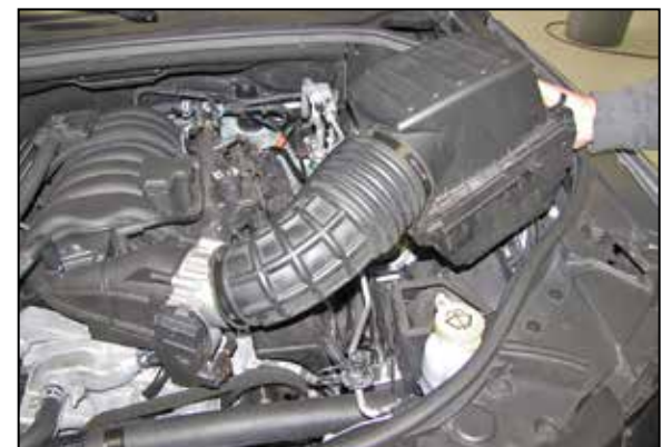
6. Lift up the air filter assembly to dislodge it from the mounting grommets and the remove the complete assembly from the vehicle. NOTE: K&N Engineering, Inc., recommends that customers do not discard factory air intake.
