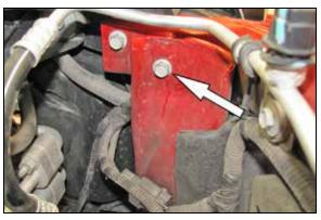
12. Remove the core support bolt shown. **NOTE: This bolt will be reused in a later step.**
