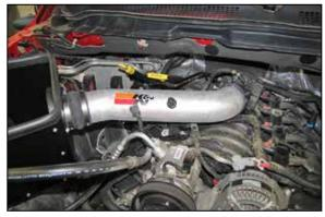
19. Install the K&N<sup>®</sup> intake tube into the coupler at the heat shield and then into the coupler at the throttle body. Adjust the tube for best fit and then secure with the provided hose clamp.
