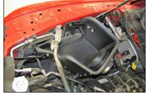
14. Install the heat shield into the vehicle and secure with the factory bolts removed in the previous steps.
