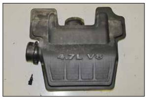
17. Remove the inlet air temperature sensor from the factory air filter housing. **NOTE: Be careful removing the inlet air temperature sensor as it is very fragile.**
