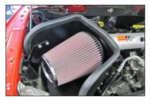
22. Install the K&N<sup>®</sup> air filter onto the adapter and secure with the provided hose clamp. NOTE: Drycharger<sup>®</sup> air filter wrap; part # RF-1020DK is available to purchase separately. To learn more about Drycharger<sup>®</sup> filter wraps or look up color availability please visit http://www.knfilters.com<sup>®</sup>.
