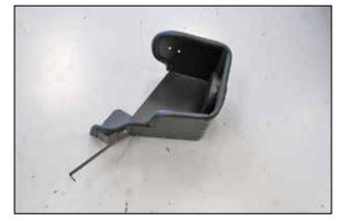
9. Install the provided heat shield mounting bracket (083103-1) onto the heat shield using the provided hardware.
