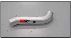
15. Install the provided grommet into the K&N $^{\mbox{\scriptsize \$}}$  intake tube as shown.
