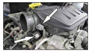
4. Disconnect the inlet air temperature sensor electrical connection and remove the bolt shown that secures the intake plenum. Lift up and remove the intake plenum from the vehicle. NOTE: K&N Engineering, Inc., recommends that
