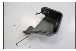
10. Install the provided heat shield mounting bracket (083127) onto the heat shield using the provided hardware.
