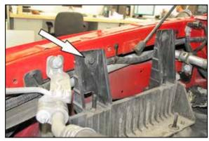
13. Remove the air filter housing mounting bracket bolt shown.
