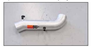
18. Remove the sealing O-ring from the sensor and then install the inlet air temperature sensor into the grommet installed into the intake tube. NOTE: Be careful installing the inlet air temperature sensor as it is very fragile.
