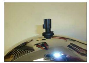
15. Remove the IAT sensor from the factory intake tube and then remove the O-Ring from the sensor. Using the provided grommet, install the sensor into the K&N intake tube as shown. **NOTE: The IAT sensor is very fragile, use caution while** handling the sensor so as not to damage it.
