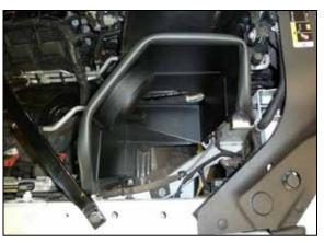
10. Install the K&N heat shield into the vehicle.
