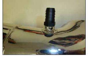
14. Install the provided vent fitting into the K&N intake tube as shown. **NOTE: NPT fitting has tapered threads and only designed to be installed until hand tight, then tighten one rotation or when the fittig becomes difficult to return.**
