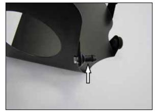
6. Install the air box mounting stud onto the K&N heat shield using the provided hardware.
