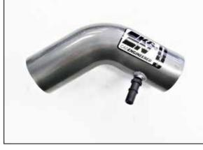
10. Install the vent fitting into the K&N intake tube as shown.
