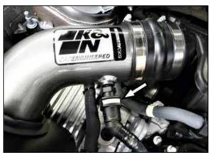
12. Connect the factory crank case vent hose to the quick connect fitting installed into the K&N intake tube.
