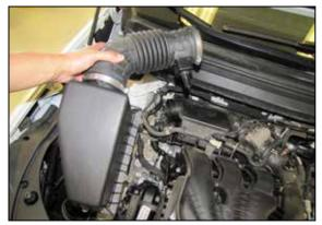
4. Loosen the hose clamp that secures the intake tube to the intake plenum. Disconnect the intake tube and then remove the complete intake system. 5. Remove the two factory mounting grommets
