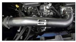
15. Install the K&N intake tube into the hump coupler and then into the step coupler at the throttle body, adjust the tube for best fit and then secure with the provided hose clamps.
