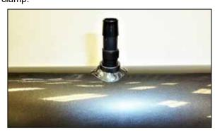
13. Install the provided CCV fitting into the K&N intake tube as shown.
