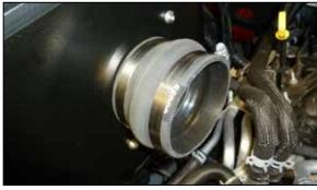
11. Install the provided hump coupler onto the filter adapter and secure with the provided hose clamp.
