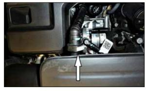
3. Depress the locking tab and then disconnect the CCV hose from the intake plenum.
