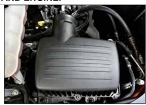
6. Pull the air filter housing straight up and remove it from the vehicle.
