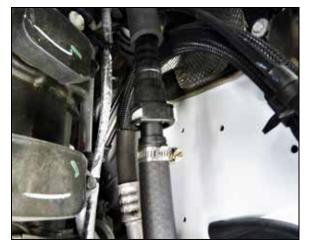
21. Connect the CCV extension to the factory CCV quick connect.
