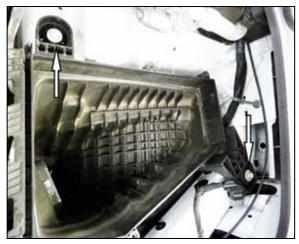
8. Remove the two bolts that secure the lower air filter housing and then remove the housing from the vehicle.
