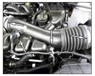
2. Remove the two bolts that secure the engine cover and then remove the cover from the vehicle.
