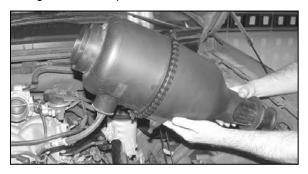
5. Pull firmly up on the air filter assembly to remove it from the mounting grommets.
