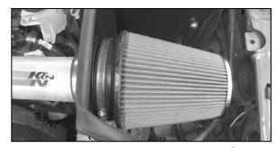
23. Install the filter assembly onto the K&N® intake tube and secure with the provided hose clamp.
