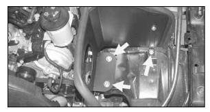
10. Install the heatshield as shown and secure with the provided hardware.
