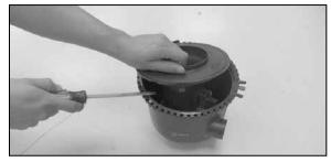
13. Using a flat blade screwdriver, push in and release the four clips that retain the mass air sensor retaining plate.
