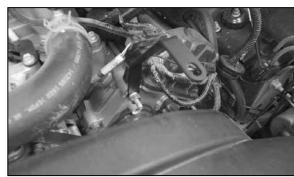
18. Install the tube mounting bracket (07198) onto the 8mm stud protruding from the engine with the factory nut, and the flat washer and wave washer provided. Do not completely tighten at this time.
