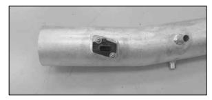
15. Install the mass air sensor assembly into the K&N<sup>®</sup> intake tube and secure with the factory mounting bolts.
