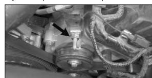
17. Remove the nut shown from the 8mm stud protruding from the engine.
