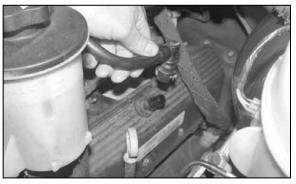
2. Rotate the crank case vent hose locking ring and pull the crank case vent hose off of the valve cover.
