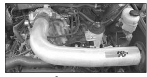
19. Install the K&N<sup>®</sup> intake tube into the silicone hose at the throttle body and align with the mounting bracket and secure with the provided hose clamp and hardware.
