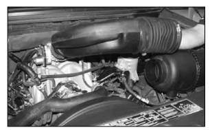
3. Loosen the stock intake tube hose clamps, and remove the intake tube from vehicle.
