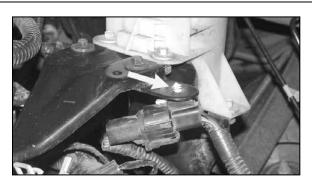
4. Unhook the secondary mass air sensor electrical connection from the power steering reservoir bracket, then unlock the electrical connection locking tabs and separate the electrical connection
