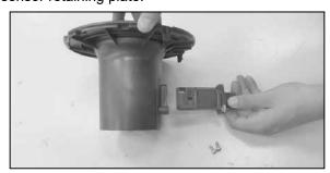
Remove the mass air sensor retaining screws and then remove the mass air sensors as shown.
