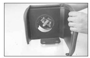
8. Install the edge trim into the hole in the heat shield as shown.
