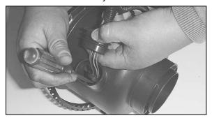
12. Slide the rubber grommet back and disconnect the primary mass air sensor electrical connection, using a flat blade screwdriver.
