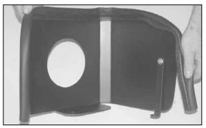
7. Install the edge trim onto the heatshield as shown. Trim if needed.
