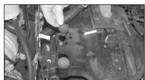
9. Install the provided nut inserts into the air box mounting holes as shown.
