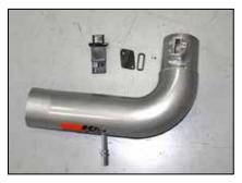
19. On vehicles that are equipped with a mass air sensor install the sensor into the K&N<sup>®</sup> intake tube and secure with the provided hardware. On all other vehicles, install the provided gasket onto the block off plate and install the block off plate into the K&N<sup>®</sup> intake tube and secure with the provided hardware.
