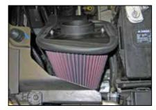
13. Flex the heat shield in on the rubber mounted studs for clearance to install the K&N<sup>®</sup> air filter. Install the air filter and secure it with the provided hose clamp.
