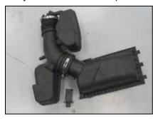
18. Remove the two screws securing the mass air sensor, then remove mass air sensor from the factory air box.
