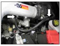
23. Connect the provided EVAP vent line to the fitting on the K&N<sup>®</sup> intake tube and then connect the open end to the factory EVAP check valve.
