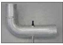
20. Install the NPT vent fitting into the K&N $^{\mbox{\tiny \$}}$  intake tube as shown.
