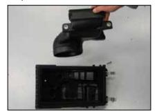
16. Remove the screw securing the fresh air intake
