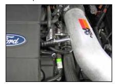
22. Connect the crank case vent hose to the  $K\&N^{\circledast}$  intake tube.
