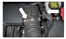
4. Loosen the hose clamp securing the factory intake tube to the throttle body and disconnect the EVAP vent line from the EVAP check valve.
