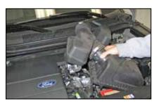
5. Release the two upper air box retaining clips and then remove the upper air box and intake tube assembly from the vehicle.
