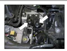
9. Install the two provided rubber mounted studs onto the air box mounting bracket as shown. NOTE: Be sure to place a fender washer on the top and bottom sides of the air box mounting bracket.
