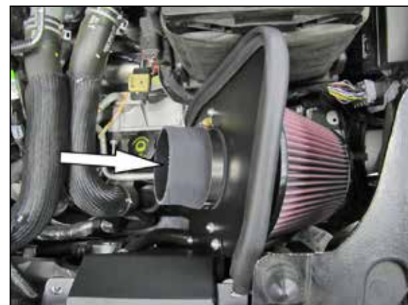
15. Install the provided silicone hose (08496) onto the filter adapter and secure with the provided hose clamp.
