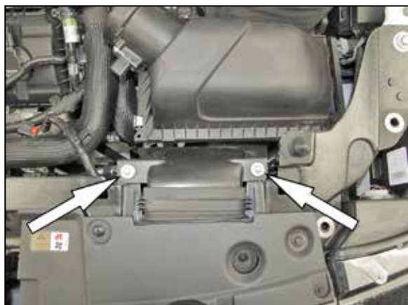
7. Remove the two bolts which secure the fresh air intake scoop.
