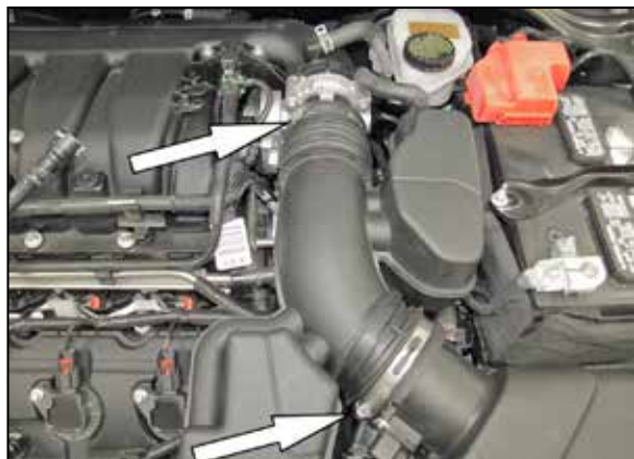
5. Loosen the two hose clamps which secure the factory intake tube to the throttle body and factory air box. Remove the factory intake tube from the vehicle.
