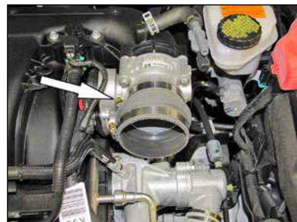
16. Install the provided silicone hose (08171) onto the throttle body and secure with the provided hose clamp.
