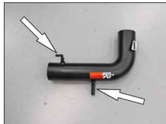
17. Install the provided 90° NPT vent fitting and NPT quick disconnect fitting into the K&N® intake tube as shown.
