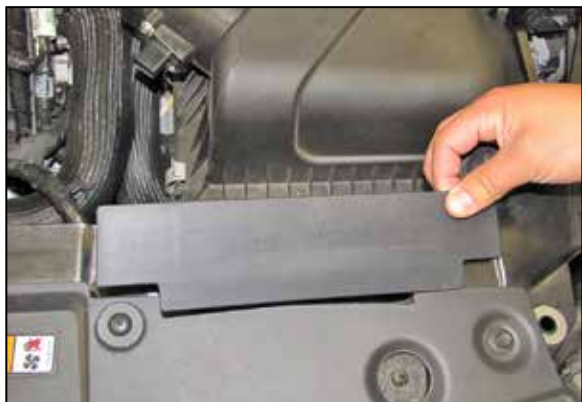
6. Remove the plastic cover over the fresh air intake scoop.
