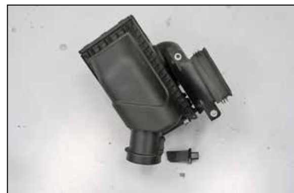
18. Remove the two screws that secure the mass air sensor into the factory air box and then remove the sensor from the air box.
