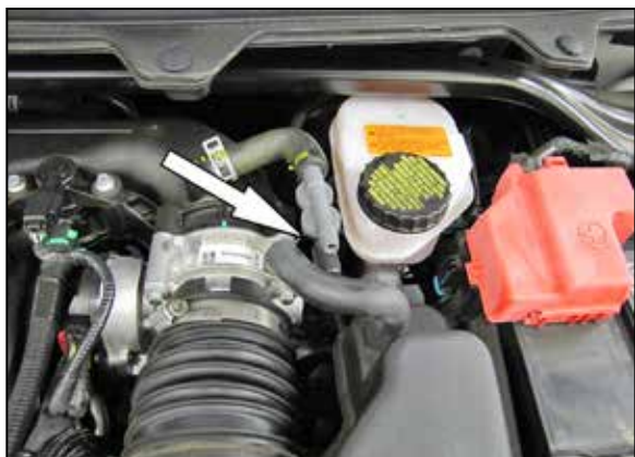
4. Disconnect the EVAP vent line from the check valve as shown.
