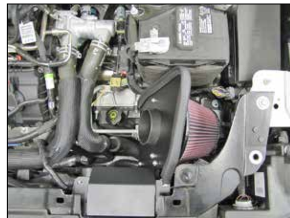
14. Install the heat shield assembly into the vehicle so that the mounting studs go into the air box mounting grommets.
