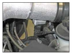
33. Connect the mass air sensor electrical connection.
