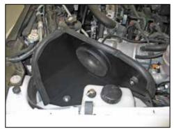
23. Install the heat shield assembly into the vehicle so the inserts align with the air box mounting grommet locations. Secure the heat shield mounting bracket to the inner fender with the coolant reservoir and spacer provided. Then secure the bottom of the heat shield to the inner fender brace with the inserted nuts.
