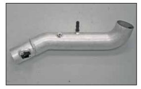
29. Install the provided quick disconnect fitting into the K&N<sup>®</sup> intake tube as shown. **NOTE: Plastic NPT fittings are easy to cross**
