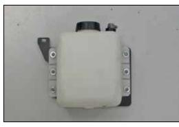
15. Attach the provided coolant reservoir bottle to mounting bracket (083144) using the provided hardware.
