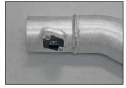
28. Install the mass air sensor into the K&N<sup>®</sup> intake tube and secure with the provided hardware.
