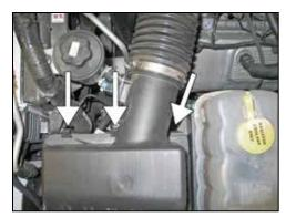
4. Release the three retaining clips on the upper air box.
