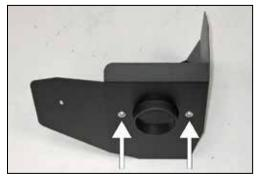
17. Install the filter adapter into the heat shield and secure with the provided hardware.
