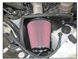
34. Mount the K&N<sup>®</sup> air filter onto the filter adapter and secure with a provided hose clamp. Transfer the coolant from the factory reservoir into the K&N<sup>®</sup> coolant reservoir.
