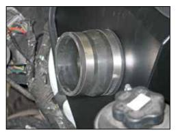
26. Install the provided silicone hose (08051) onto the filter adapter and secure with the provided hose clamp.
