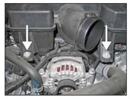
9. Remove the two bolts that secure the intake plenum to the intake manifold.
