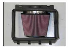
13. Install the K&N<sup>®</sup> air filter onto the filter adapter and secure with the provided hose clamp.
