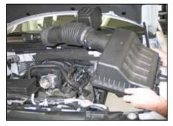
6. Remove the upper airbox housing and intake tube assembly from the vehicle. **NOTE: K&N Engineering, Inc., recommends that customers do not discard factory air intake.**  8. Remove the center upper airbox retaining clip from the lower airbox.
