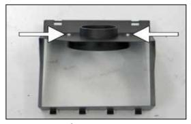
9. Install the K&N<sup>®</sup> filter adapter into the heat shield as shown. Secure with the provided hardware.
