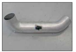
18. Install the mass air sensor into the  $K\&N^{\mathbb{R}}$  intake tube as shown, secure with the provided hardware.
