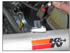
22. Connect the provided mass air sensor extension harness into the factory connector and then connect the open end to the mass air sensor electrical connection.
