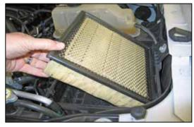
7. Remove the air filter from the lower airbox.
