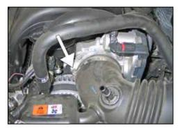
4. Loosen the hose clamp that secures the intake tube to the throttle body.
