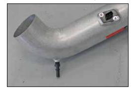
19. Install the provided crankcase vent fitting into the K&N<sup>®</sup> intake tube as shown.
