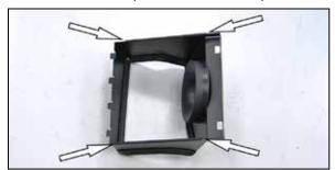
10. Install the two 9" sections of edge trim onto the bottom of the heat shield as shown.
