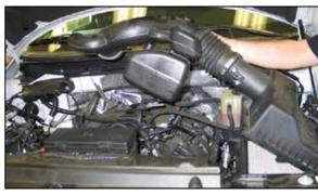
6. Release the three clips securing the upper air box housing to the lower housing and then remove the intake tube/upper airbox and air filter from the vehicle.
