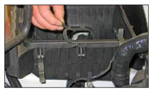
12. Remove the center airbox retaining clip.
