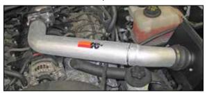
19. Install the K&N® intake tube into the silicone hose at the air filter and then into the silicone hose at the throttle body and secure with the provided hose clamps.
