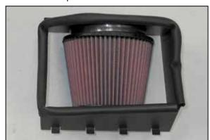
11. Install the K&N® air filter onto the filter adapter and secure with the provided hose clamp.
