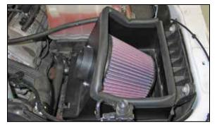
13. Install the K&N® filter/heat shield assembly and secure with the two remaining factory upper air box retaining clips.
