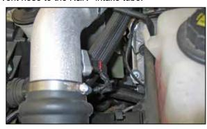
21. Reconnect the mass air sensor electrical connection.
