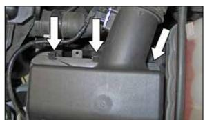
3. Release the three upper air box retaining clips.
