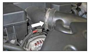
4. Loosen the hose clamp securing the intake tube to the intake plenum.
