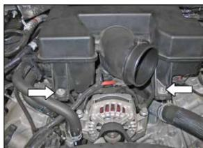
7. Remove the two bolts securing the intake plenum to the intake manifold and then loosen the hose clamp securing the plenum to the throttle body.
