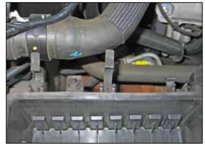
12. Remove the center upper air box retaining clip from the lower air box.
