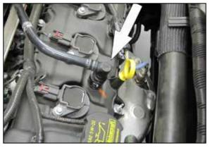
5. Rotate the locking tab and then disconnect the crank case vent tube from the valve cover.
