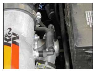
21. Using the provided 3/8" hose, connect the EVAP vent line to the 90° fitting installed into the K&N® intake tube.
