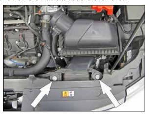
8. Remove the two bolts securing the fresh air intake scoop to the core support.
