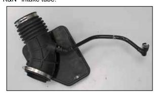
22. Rotate the locking tab and then remove the crank case vent line from the factory intake tube assembly.
