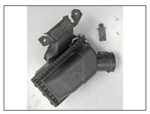
16. Remove the two screws securing the mass air sensor into the factory air box and then remove the mass air sensor from the air box.
