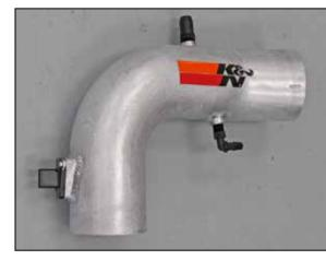
17. Install the mass air sensor into the K&N<sup>®</sup> intake tube and secure with the provide hardware.
