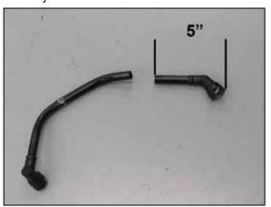
23. Measure 5" from the intake tube end of the crank case vent tube and then cut the crank case vent tube as shown.
