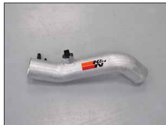
17. Install the mass air sensor into the K&N® intake tube and secure with the hardware provided.
