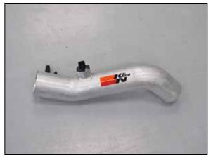
17. Install the mass air sensor into the K&N® intake tube and secure with the hardware provided.
