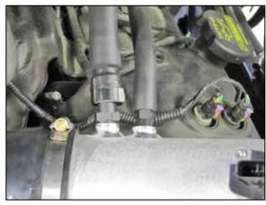
19. Connect the EVAP vent line and crank case vent lines to the fittings installed into the K&N® intake tube.
