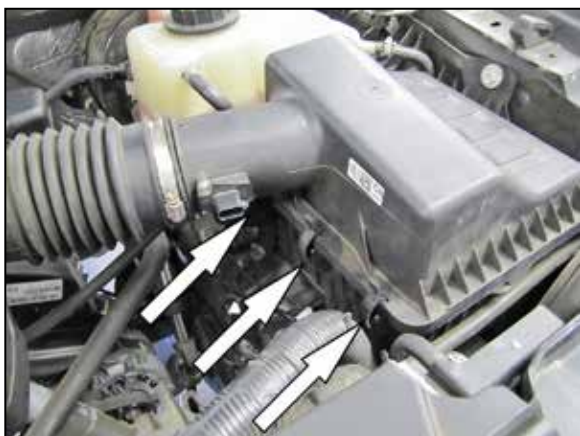
5. Release the three clips securing the upper air box housing to the lower air box housing. Then remove the stock intake tube/upper air box housing and air filter from the vehicle.
