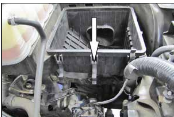
6. Remove the center upper air box retaining clip from the lower air box housing. NOTE: K&N Engineering, Inc., recommends that customers do not discard factory air intake.
