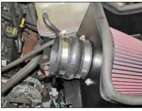
14. Install the provided hump hose (084057) onto the filter adapter and secure with the provided hose clamp.
