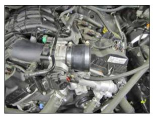
7. Install the provided silicone hose (08724) onto the throttle body and secure with the provided hose clamp.
