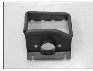
9. Install the provided filter adapter into the heat shield and secure with the provided hardware.
