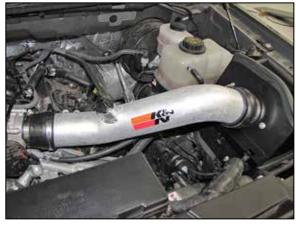
18. Install the K&N® intake tube into the silicone hose at the throttle body and then into hump hose at the filter adapter. Then secure with the provided hose clamps.
