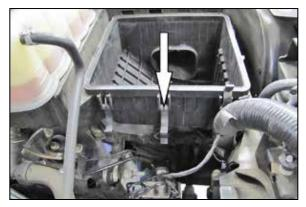
6. Remove the center upper air box retaining clip from the lower air box housing.
