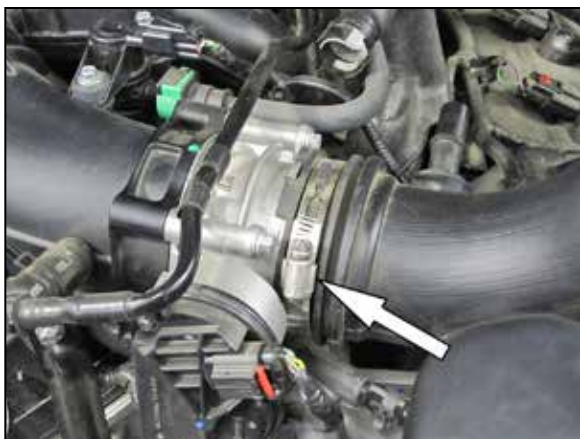
4. Loosen the hose clamp securing the stock intake tube the throttle body.
