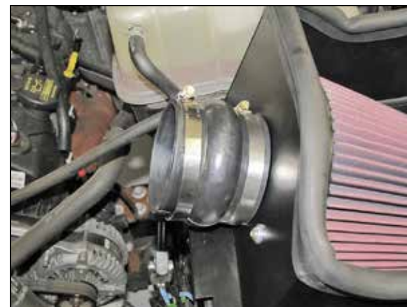
14. Install the provided hump hose (084057) onto the filter adapter and secure with the provided hose clamp.
