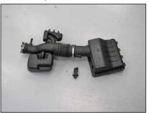
16. Remove the mass air sensor from the stock upper air box housing.
