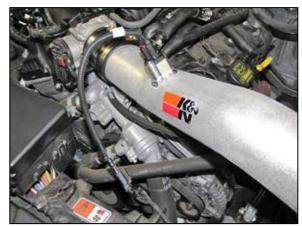
20. Connect the provided mass air extension harness into the factory wiring harness and then connect the other end onto the mass air ser
