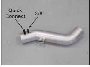
15. Install the Quick connect and 3/8" vent fitting into the K&N<sup>®</sup> intake tube as shown. NOTE: Plastic NPT fittings are easy to cross
