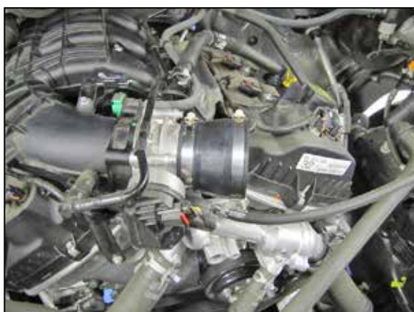
7. Install the provided silicone hose (08724) onto the throttle body and secure with the provided hose clamp.
