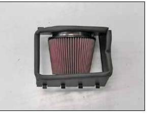
12. Install the K&N<sup>®</sup> air filter onto the filter adapter and secure with the provided hose clamp.
