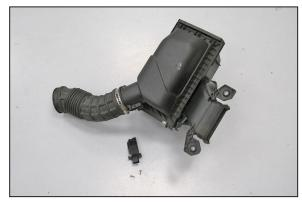
14. Remove the two screws securing the inlet air temperature sensor into the factory intake tube and then remove the sensor.
