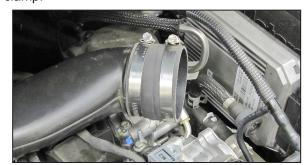
13. Install the provided coupling hose (08711) onto the turbo inlet tube and secure with the provided hose clamp.
