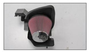
10. Install the K&N® air filter onto the filter adapter and secure with the provided hose clamp.
