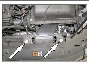
5. Remove the two bolts that secure the fresh air intake to the core support and then lift up and remove the complete intake assembly.
