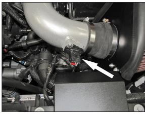
17. Reconnect the inlet air temperature electrical connection.
