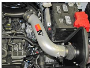
16. Install the K&N® intake tube into the hose at the throttle body and then into the hose at the filter adapter, align the tube for best fit and then secure with the provided hose clamps.
