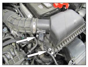
3. Disconnect the inlet air temperature sensor electrical connection and unhook the harness from the air box.
