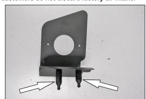
6. Install the two provided stand offs onto the heat shields using the provided hardware.
