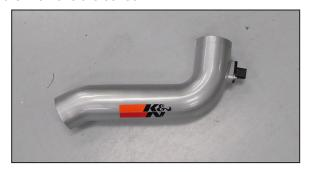
15. Install the inlet air temperature sensor into the K&N® intake tube and secure with the hardware provided.
