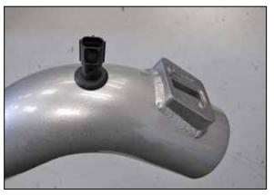
14b. On vehicles equipped with the later style sensor, install the provided grommet and factory sensor into the hole drilled in the previous step.
