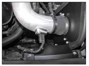
18. Reconnect the inlet air temperature sensor electrical connection.
