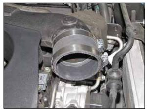
16. Install the appropriate coupling hose onto the turbo inlet pipe and secure with the provided hose clamp.
