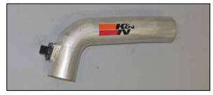
14. On vehicles equipped with the early style inlet temperature sensor, install the sensor into the K&N<sup>®</sup> intake tube and secure with the hardware provided.
