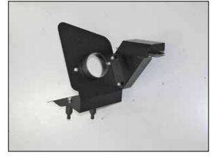
8. Secure the provided fresh air intake scoop to the heat shield using the provided hardware. NOTE: Do not completely tighten the scoop at this time.
