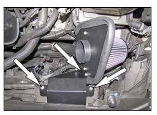
12. Secure the fresh air intake scoop to the core support and tighten the bolts which secure the scoop to the heat shield.
