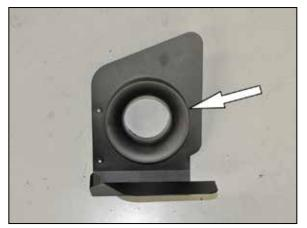
6. Secure the air filter adapter to the heat shield using the provided hardware.
