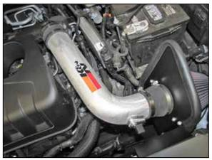
17. Install the K&N<sup>®</sup> intake tube assembly into the coupler at the turbo inlet tube, then slide the step coupler onto the filter adapter. Adjust the tube for best fit and secure the hose clamps.
