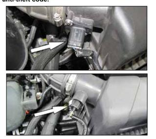
2. Release the locking tab and then disconnect the inlet air temperature sensor electrical connection and unhook the harness from the air filter housing. NOTE: there is two different style inlet air temperature sensors used throughout the year coverage.
