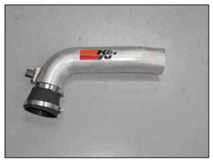
15. Install the step coupler hose (084055) onto the K&N<sup>®</sup> intake tube as shown. Do not tighten the hose clamp at this time.
