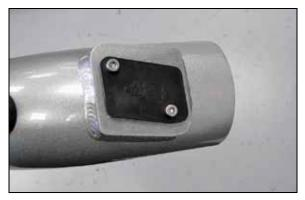
14c. Install the sensor block off plate with the provided gasket using the hardware provided.
