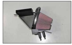
10. Install the air filter onto the filter adapter and secure with the provided hose clamp. NOTE: Drycharger<sup>®</sup> air filter wrap; part # RF-1048DK is available to purchase separately.
