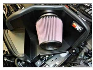
17. Install the K&N air filter and secure with the provided hose clamp.
