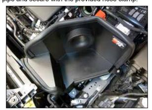
11. Install the heat shield assembly into the vehicle so the mounting studs insert into the factory air filter housing mounting grommets.
