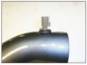
14. Using the provided grommet, install the IAT sensor into the K&N intake tube.
