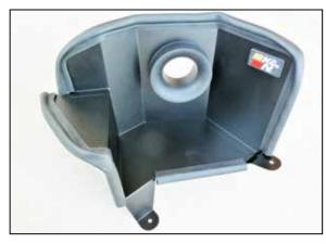
7. Install the filter adapter into the heat shield and secure with the provided hardware. Install the K&N badge onto the heat shield and secure with the locking plate.
