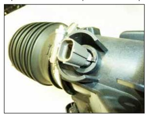
13. Lift the locking tab and then rotate the IAT sensor counterclockwise to remove it from the factory air filter housing and then remove the O-ring from the sensor.
