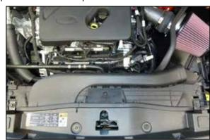
18. Reinstall the fresh air intake duct and secure with the factory push pins.
