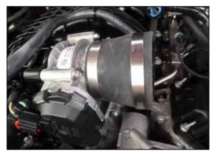
11. Install the provided step coupler onto the throttle body and secure with the provided hose clamp.
