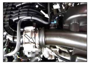
2. Loosen the hose clamp that secures the factory intake tube to the throttle body and then release the vent line quick connector and separate the vent line from the intake tube.
