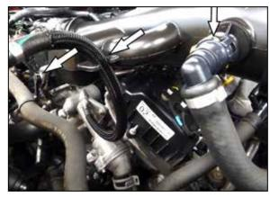
3. Unhook the coolant hose from the intake tube and separate the hose hanger. On models equipped with the vent hose, release the quick connect fitting and separate the vent hose from the intake tube.
