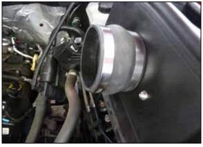
10. Install the provided hump coupler onto the adapter and secure with the provided hose clamp.
