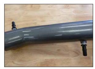
12. Install the provided quick connect vent fittings into the K&N intake tube. On models that are equipped with one vent line, install the provided 3/8npt plug into the unused vent port.
