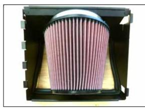
8. Install the K&N air filter onto the adapter and secure with the provided hose clamp.
