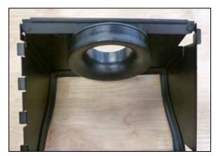
7. Install the provided filter adapter into the heat shield as shown using the provided hardware.
