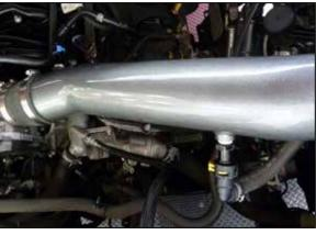
14. Connect the factory vent line(s) to the fitting(S) installed into the K&N intake tube.
