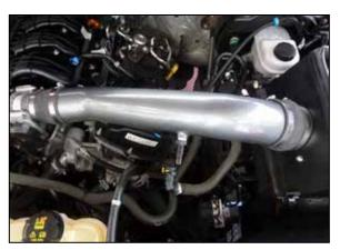
13. Install the K&N intake tube into the couplers and adjust for best fit. Then secure the provided hose clamps.
