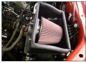
9. Install the heat shield/filter assembly onto the lower air filter housing and secure with the factory retaining clips.
