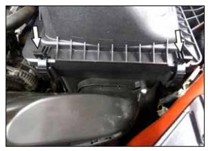
4. Release the two clips that secure the upper filter housing and then remove the upper housing, intake tube and factory air filter.
