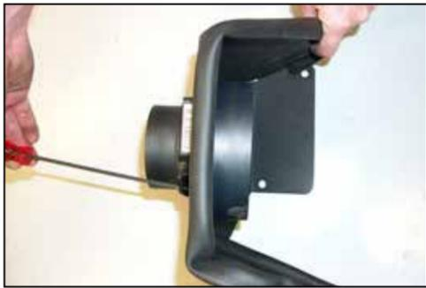
11. Using the provided hardware assemble the mass air adapter, heat shield, gaskets and the stock mass air sensor as shown.
