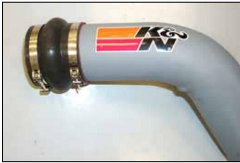
15. Install the silicone step hump hose and hose clamps onto K&N® intake tube as shown.
