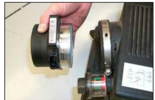
7. Loosen the hose clamp on the air cleaner then remove the mass air sensor as shown.
