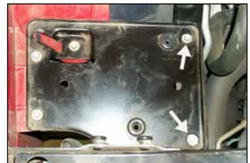
8. Remove the two stock air cleaner support tray bolts as shown.
