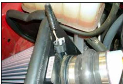
19. Reconnect the mass air sensor electrical connection as shown.
