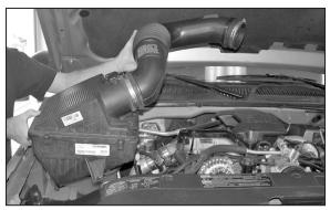
4. Lift up on the air box assembly to release from the mounting grommets, and then remove the air box and intake tube assembly from the vehicle.
