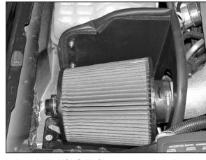
19. Install the K&N® Air filter onto intake tube as shown then tighten completely.
