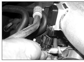
20. Reconnect the mass air sensor electrical connection as shown.
