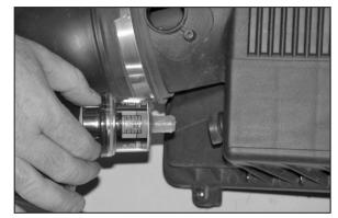
13. Remove the restriction gauge and grommet from the stock air box as shown.
