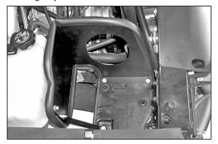
11. Mount the heat shield onto the airbox mounting tray and secure with the three bolts removed in step 10.
