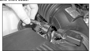
2. Depress the locking tab on the mass air sensor electrical connector, and then disconnect the electrical connection.
