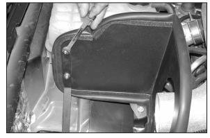
16. Adjust heat shield and bracket for necessary clearance, then tighten all hardware completely.
