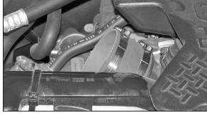
5. Install the silicone hose (08456) onto the intake manifold and secure with the provided hose clamps.
