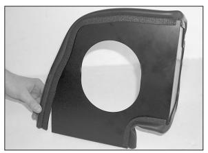
8. Apply the provided trim seal to the heat shield assembly as show. Trim if necessary.
