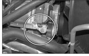
6. Remove the lower front engine processor mounting bolt shown.
