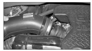
3. Loosen the hose clamp, which secures the intake tube to the intake manifold, and then disconnect the intake tube from the intake manifold.
