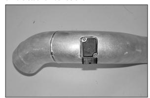
14. Install the mass air sensor into the K&N® intake tube and secure with the provided hardware as shown.
