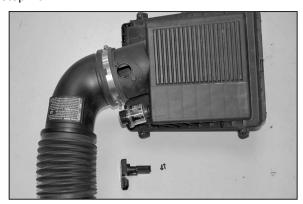
12. Using the "TORX" T20 wrench provided, loosen and remove the two-torx screw that retain the mass air sensor, and then remove the sensor.
