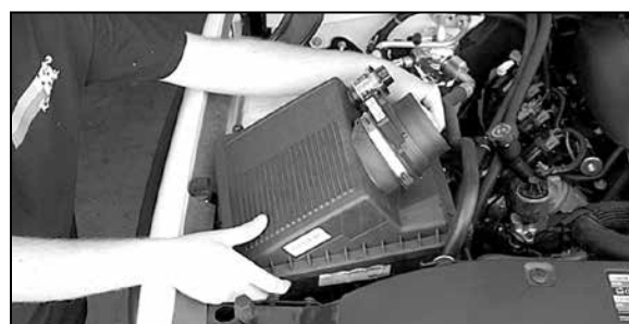
4. Pull firmly upwards to release the air cleaner assembly from the mounting tray grommets, then remove the assembly. NOTE: K&N Engineering, Inc., recommends that customers do not discard factory air intake.
