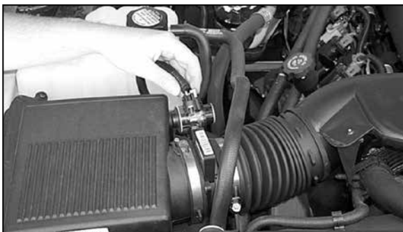
2. Disconnect the mass air sensor electrician connection.
