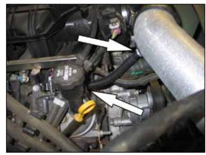
19. Connect the provided crank case vent hose the fitting installed into the K&N® intake tube and then connect the open end to the valve cover port.
