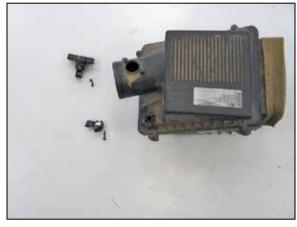
15. Remove the screws securing the mass air sensor and pressure sensor into the factory air box lid and then remove the sensors.
