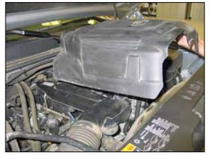
3. Lift up and remove the engine cover as shown.
