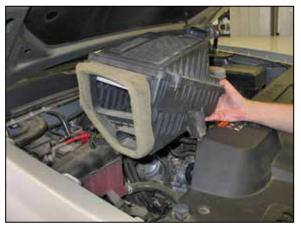
8. Lift up and remove the factory air box from the vehicle.
