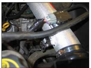
20. Connect the mass air sensor and pressure sensor electrical connections.
