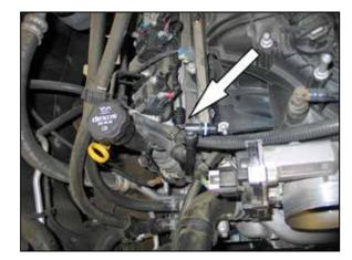
7. Rotate the crank case vent hose counter clockwise to access the retaining clip on the valve cover, release the clip and then remove the hose from the valve cover port.
