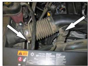
6. Loosen the hose clamp securing the intake tube to the air box housing and disconnect the radiator hose retaining clip from the intake tube. Then remove the intake tube from the vehicle.
