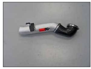
17. Install the provided angle hose onto the K&N® intake tube as shown.
