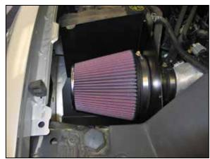
21. Install the K&N® air filter and secure with the provided hose clamp.
