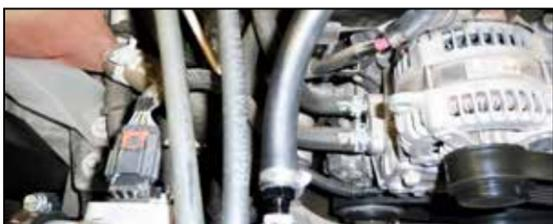
20. Connect the passenger side CCV hose to the K&N intake tube and secure with the provided hose clamps. Reconnect the mass air sensor electrical connection.
