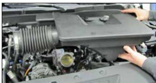
5. Remove the intake plenum from the vehicle.
