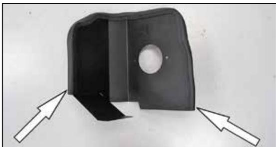
8. Install the provided edge trim onto the heat shield as shown.
