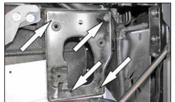
7. Remove the four bolts securing the air box mounting tray and then remove the tray from the vehicle.
