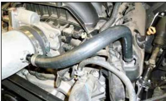
19. Install the provided CCV hoses onto the valve cover ports and connect the driver side hose to the K&N intake tube and secure with the provided hose clamps.
