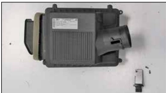
15. Remove the mass air sensor from the factory air box.
