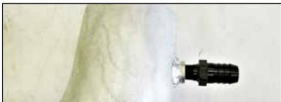
17. Apply thread sealant to the remaining CCV fitting and install it into the K&N intake tube.
