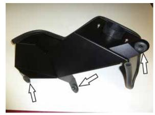
5. Remove the three factory mounting grommets from the factory air filter housing and install them into the K&N heat shield as shown.
