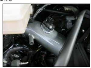
22. Remove the mass air sensor from the factory air filter housing and install it into the K&N intake tube using the provided screws.
