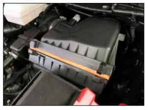
3. Release the two clips that secure the upper air filter housing.
