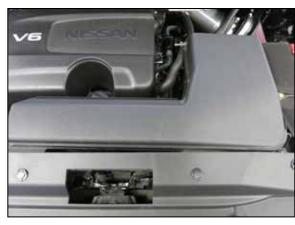
28. Reinstall the factory fresh air intake duct and secure with the factory hardware.
