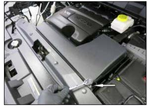
2. Remove the two bolts that secure the fresh air duct to the core support and then remove the duct from the vehicle.
