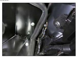
19. Align the mounting bracket with the ground location and then secure the bracket with the factory bolt removed from the ground. Be sure the ground is between the bracket and the strut tower, the ground should be in its original location.
