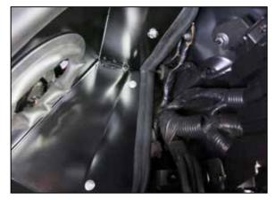
20. Secure the heatshield to the mounting studs with the provided hardware.
