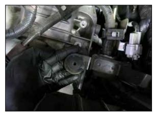
10. The  $\frac{1}{2}$ " and 1" rubber mounted studs will be assembled in the order shown onto the air filter housing mounting points.
