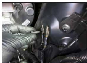
17. Remove the bolt that secures the ground to the strut tower, do not remove the ground.
