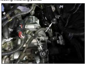
11. Install the  $\frac{1}{2}$ " rubber mounted stud onto the front housing mount and the 1" mounting stud onto the rear housing mount.
