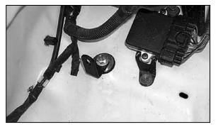
14. Install the "L" bracket onto the existing air boxmounting hole.
