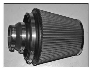
25. Install the silicone hose (084093) onto the air filter assembly as shown and secure with the provided hose clamps.
