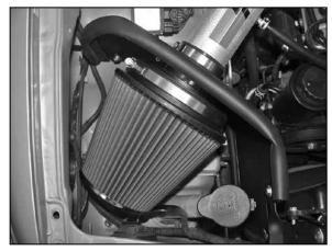
26. Install the air filter assembly onto the K&N<sup>®</sup> intake tube and secure with the provided hose clamp.
