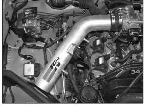
19. Install the K&N<sup>®</sup> intake tube onto the throttle body and align with the tube mounting bracket installed in step #16. Secure the tube with the provided hardware to the mounting bracket and tighten the hose clamp at the throttle body. 23. On vehicles equipped with crank case vent resonator, connect the factory crank case vent hose onto the resonator as shown.
