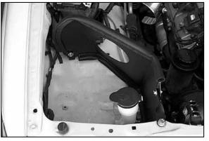
17. Install the heat shield and secure it to the new K&N<sup>®</sup> brackets with the hardware provided as shown. Do not tighten completely.
