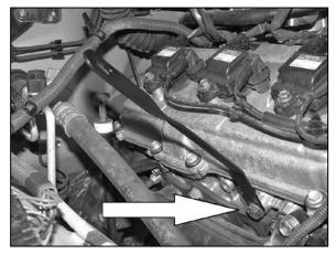
16. Install the tube-mounting bracket onto engine with the supplied hardware as shown. NOTE: The bracket will bolt to the threaded boss next in the cylinder head next to the power steering pump bracket.
