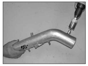
8. On vehicles equipped with the crank case resonator chamber, using a 1-3/8" hole saw, drill out the 5/8" vent port as shown. NOTE: Be sure to remove any burrs in the hole after drilling.
