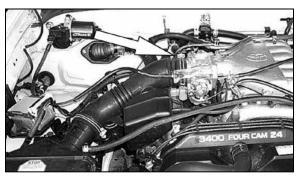
4. Loosen the hose clamps at the throttle body.
