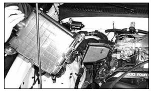
6. Remove the complete air intake system. NOTE: K&N Engineering, Inc., recommends that customers do not discard factory air intake.
