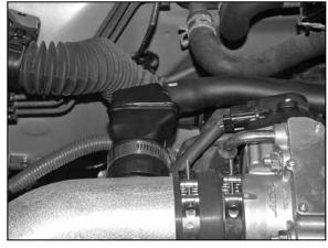
13. Install the two pieces of edge trim onto the heat shield as shown above.
