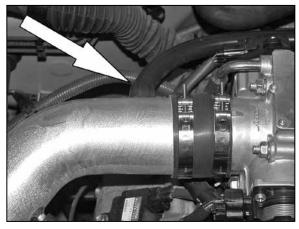
22. On vehicles not equipped with the crank case vent resonator, attach the provided silicone hose onto the crankcase vent and secure with the provided hose clamp. Then connect it to the K&N<sup>®</sup> intake tube as shown.
