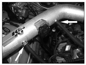
20. Install the provided silicone hose onto the engine and connect it to the  $K\&N^{\otimes}$  intake tube as shown. Then attach the vent line from EVAP canister to the  $K\&N^{\otimes}$  intake tube as shown.
