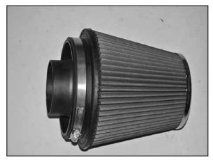
24. Install the air filter adapter into the air filter as shown.
