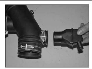
7. On vehicles equipped with the crank case vent resonator chanber, loosen the hose clamp which secures the chanber to the intake tube and remove the chamber from the tube as shown.
