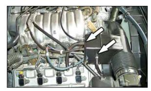
7. Disconnect the four rubber hoses from the engine as shown by the arrows. NOTE: Some '03 models may come equipped with only three vacuum lines.
