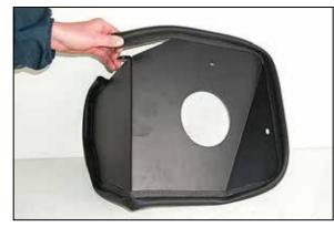
11. Apply the edge trim to the K&N<sup>®</sup> heat shield as shown above, trim if needed.
