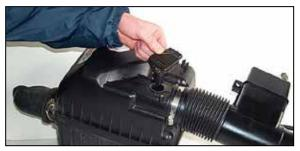
9. Loosen and remove the two screws that secure the mass-air sensor, then remove the mass-air sensor.
