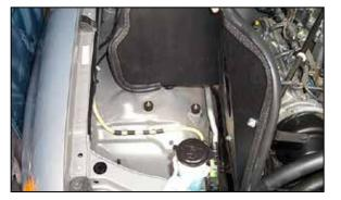
15. Install the heat shield onto the rubber mounted studs as shown above.
