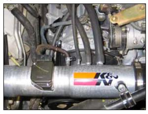
23. Install the one factory P/S vent line, crank case vent line, EVAP vent line, and fuel pressure vent line onto the K&N<sup>®</sup> intake as shown. NOTE: Some vehicles may not come with the **EVAP** vent line.
