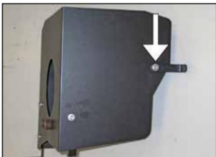
14. Install the provided heat shield mounting bracket (070742A) onto the heat shield using the provided hardware and spacer as shown.
