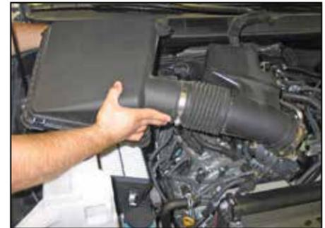
8. Remove the upper airbox/intake hose assembly from the vehicle.
