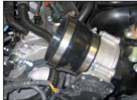
23. Install the provided silicone hose (08050) onto the throttle body as shown, secure with the provided hose clamp.
