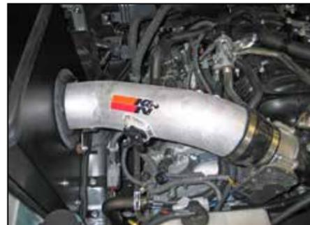
24. Install the K&N® intake tube into the silicone hose at the throttle body and align with the mounting bracket attached to the heat shield. Secure the intake tube with the provided hardware and hose clamp.
