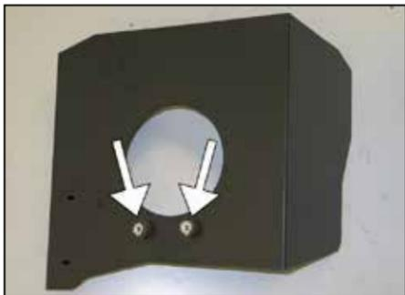
11. Install the two rubber mounted studs onto the heat shield using the provided hardware as shown.
