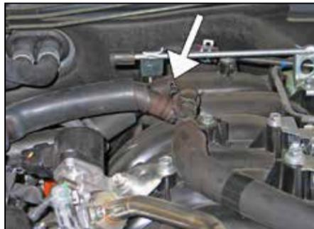
4. Disconnect the crankcase vent hose from the TEE fitting on top of the intake manifold plenum.
