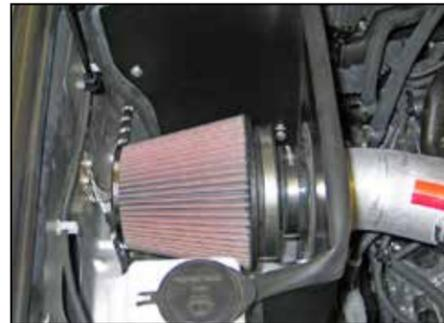
27. Install the filter assembly onto the K&N® intake tube and secure with the provided hose clamp.
