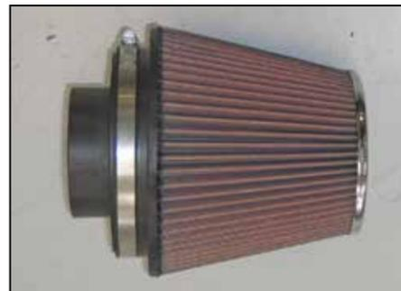
25. Install the provided filter adapter into the K&N® air filter and secure with the hose clamp.
