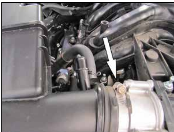
4. Loosen the hose clamp securing the factory intake tube to the throttle body.
