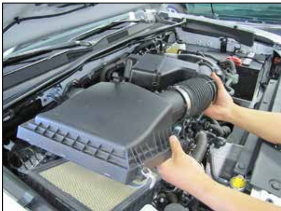
6. Release the two clips securing the air filter housing and then remove the intake tube and air filter hosing along with the factory air filter.
