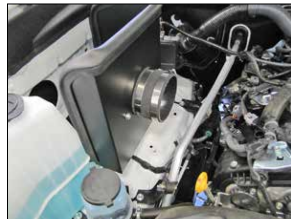
14. Install the provided step coupler (08496) onto the filter adapter and secure with the provided hose clamp.
