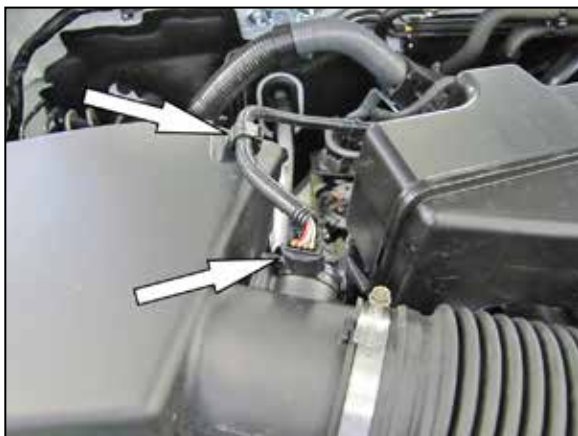
5. Disconnect the mass air sensor electrical connection and unhook the harness from the air filter housing.
