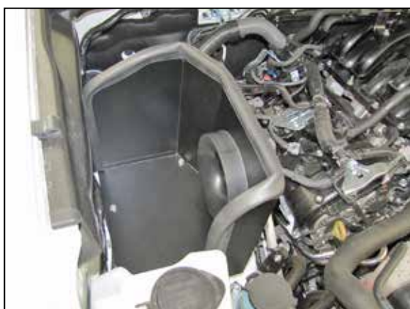
12. Install the heat shield onto the rubber mounted studs installed in the earlier step and secure with the provided hardware.
