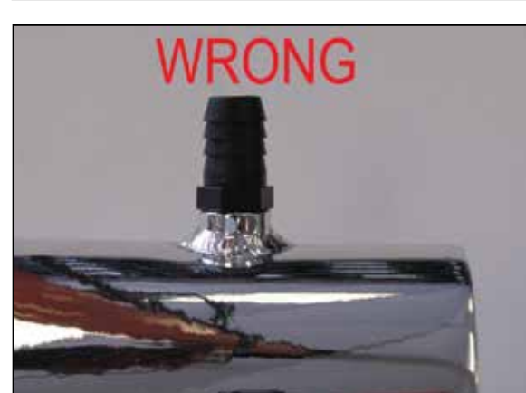
17. Install the provided vent fitting "hand" tight, then tighten 1-1/2 rotations into the K&N intake tube as shown. Do not bottom out fitting. WARNING: NPT fitting has tapered threads and only designed to be installed until hand tight, then tighten one rotation or when the fitting becomes difficult to return.
