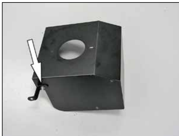
9. Install the provided heat shield bracket (07958) onto the K&N® heat shield as shown.
