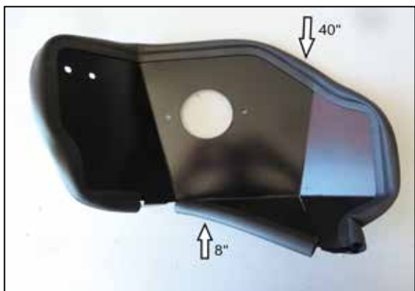
7. Cut the provided edge trim into sections of 8" & 40". Install the edge trim onto the heat shield as shown.
