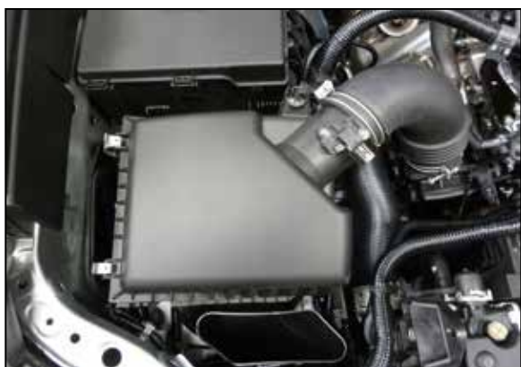
5. Lift the complete intake system straight up and remove it from the vehicle.
