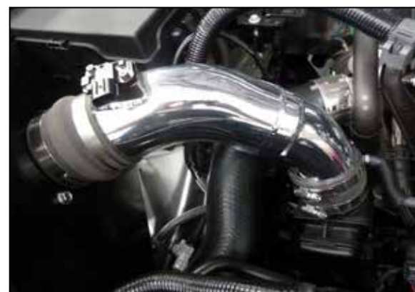
14. Install the K&N intake tube into the couplers, adjust the tube for best fit and secure with the provided hose clamps.
