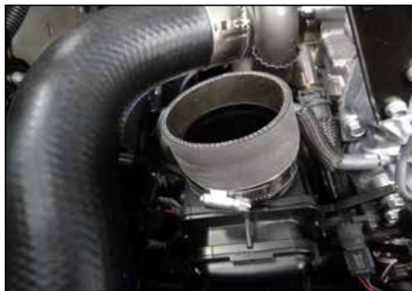
11. Install the provided straight coupler onto the plenum and secure with the provided hose clamp.
