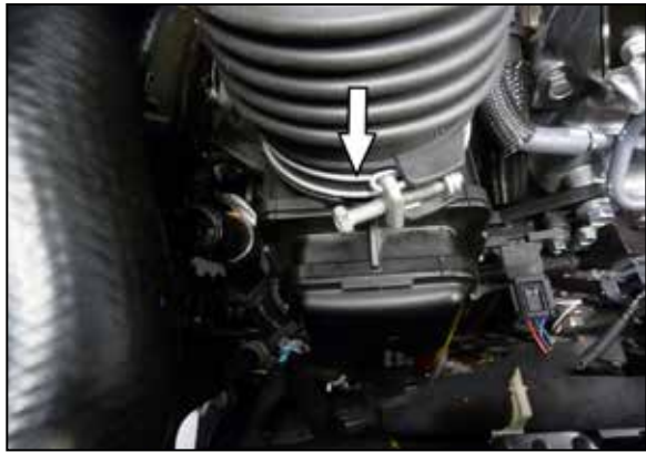
4. Loosen the hose clamp that secures the intake hose to the intake plenum.
