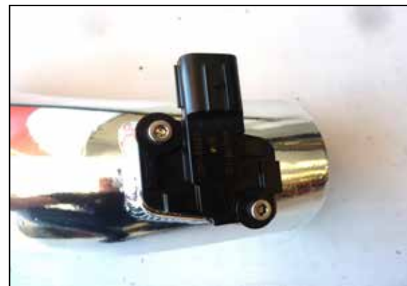
13. Remove the mass air sensor from the factory housing and install it into the K&N intake tube using the provided hardware.
