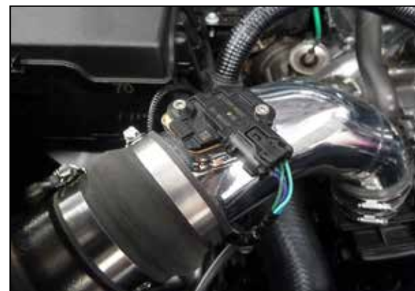
15. Connect the mass air sensor electrical connection.
