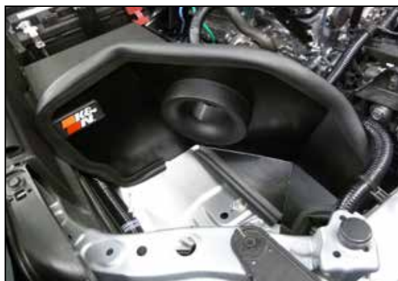
10. Install the heat shield into the vehicle and secure to the factory air box mounting locations with the provided hardware.
