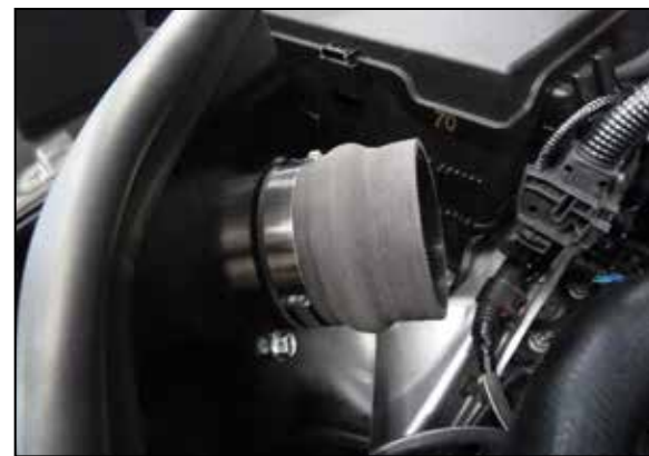
12. Install the provided hump coupler onto the filter adapter and secure with the provided hose clamp.
