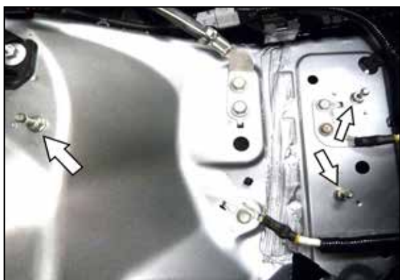
6. Remove the three airbox mounting posts.
