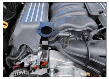
3. Slide bracket on to existing stud. Use supplied nut and washer and tighten.
