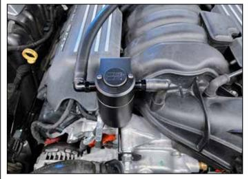
5. Insert the short barbed fitting into the manifold boot first. Then mount the Oil separator to the mounting bracket using supplied screws and lock washers. Then insert the long hose with barb into rear boot.
