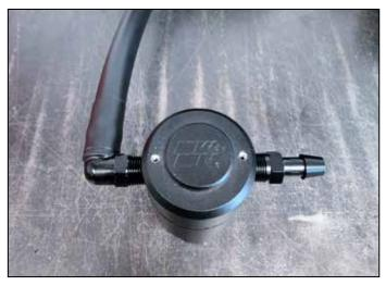
4. Assemble the hose fittings to the top of the air/oil separator. Assemble the long hose on the passenger side going to PCV valve. Assemble straight barb fitting to existing 90 degree elbow going to intake manifold. We recommend using PTFE tape on the fittings to ensure a proper seal.
