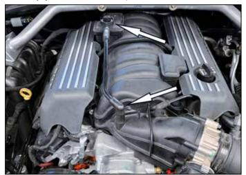
2. Remove the factory PCV hardline from both rubber connection points. You may need to twist the rubber ends with pliers to break seal on connections.
