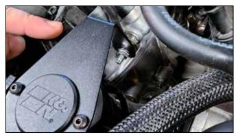
5. Mount the bracket by using the existing M6 stud on passenger cylinder head and supplied M6 flange nut.
