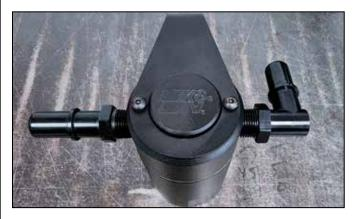
4. Assemble the quick disconnect fittings to the top of the air/ oil separator as shown. Mount the straight quick disconnect on the passenger side and the 90 degree on the driver side. We recommend using PTFE tape on the fittings to ensure a proper seal. Mount the canister to the bracket using the two button head screws and lock washers.
