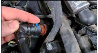
3. Remove factory PCV line by pulling tabs and removing it from the PCV valve and intake manifold. Then remove the harness retainer off the stud.
