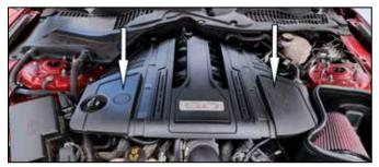
2. Remove engine cover by removing plastic caps covering (2)10mm nuts, and pull up on cover.
