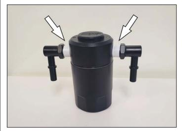
7. Assemble the quick disconnect fittings to the top of the air/oil separator. It is required to use Teflon tape on the fittings to ensure a proper seal. **NOTE: DO NOT over-tighten fittings in top of oil separator.** Mount the canister to the bracket using the two button head screws and lock washers.
