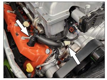
3. Remove factory PCV line by pulling tabs and removing it from the PCV valve and intake manifold
