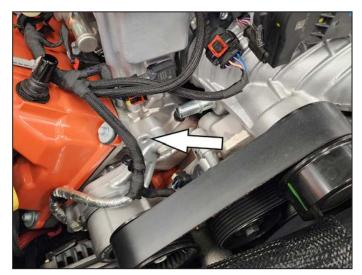
4. Remove factory wire harness holder by gently pulling towards the front of the vehicle.
