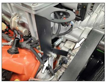
5. Mount the bracket by using the existing M10 below intake manifold connection using supplied nut. Use 1/4-20 hex head bolt, washer and nut through middle hole where wire harness holder was as shown.
