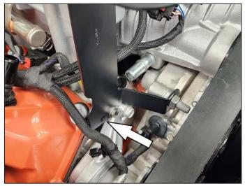
6. Plug wire harness holder in hole on the bracket.
