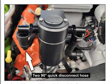
8. Install hose with straight quick disconnect between intake manifold and canister. Mount hose with two 90 degree quick disconnects between the valve cover and canister.
