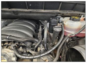
**6b. 6.2L Models** Install short hose from passenger side of oil separator to connection on driver's side cylinder head. Then install the I onger hose from driver's side of oil separator to throttlebody connection.
