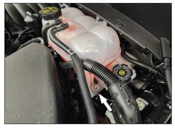
3. Remove the bolt from the coolant reservoir as shown. Gently pull the reservoir off and away from the mounting studs.
