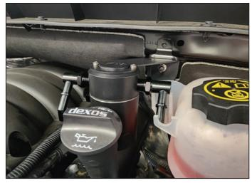
5. Mount the bracket on the passenger side coolant reservoir stud using supplied M6 nut (shown in Figure). Then mount the coolant reservoir back on studs and install mounting bolt.
