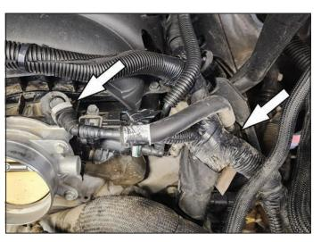
2b. **6.2L Models** Remove factory PCV line by depressing grey button and removing it from the PCV valve and intake manifold.
