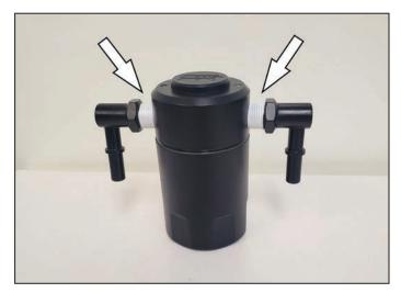
4. Assemble the quick disconnect fittings to the top of the air/oil separator. It is required to use Teflon tape on the fittings to ensure a proper seal. **NOTE: DO NOT over-tighten fittings in top of oil separator.** Mount the canister to the bracket using the two button head screws and lock washers.
