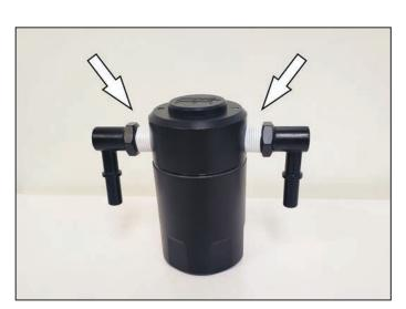
5.Assemble the quick disconnect fittings to the top of the air/oil separator. It is required to use Teflon tape on the fittings to ensure a proper seal. **NOTE: DO NOT over-tighten fittings in top of oil separator.** Mount the canister to the bracket using the two button head screws and lock washers.
