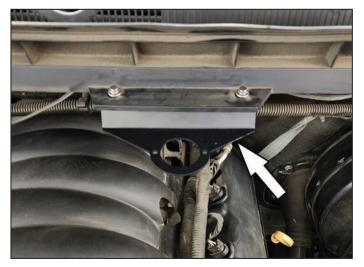
4. Mount the bracket using the 2 holes on the cowling with M6 bolts and nuts.
