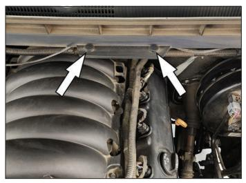
3. Remove plugs from the cowling holes.
