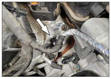
4. Remove the wire harness tab on the passenger side cylinder head by gently pulling out (threads must be clear for mounting bolt). Loosely mount the bracket by using the M8 bolt and washer behind the bracket. Once in place, perform final torque.
