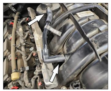
3. Remove the factory PCV hardline from both rubber connection points. You may need to twist the rubber ends with pliers to break seal on connections. Rotate the front connection 180 degrees towards the front of the vehicle.
