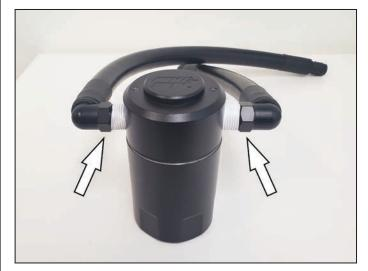
5. Assemble the hose fittings to the top of the air/oil separator. Assemble the short hose on the driver side of the canister. Assemble the long hose on the passenger side. It is required to use Teflon tape on the fittings to ensure a proper seal. **NOTE: DO NOT over-tighten fittings in top of oil separator.** Mount the canister to the bracket using the two button head screws and lock washers.
