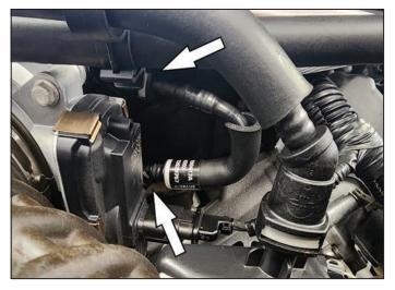
2. Remove factory PCV line by depressing grey button and removing it from the PCV valve and intake manifold.
