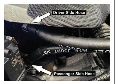
5. Install hose from passenger side of oil separator to the lower manifold connection. Install hose from driver's side of oil separator to the upper intake manifold connection. Mount the short hose to the intake manifold.
