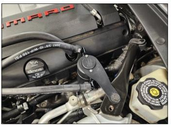
4. Mount the bracket by removing strut brace bolt closest to the firewall (shown in Figure), then mount the bracket using the existing bolt. NOTE: Vehicles equipped with a strut bar will need to uninstall prior to mounting the oil separator.
