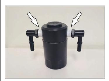
3. Assemble the quick disconnect fittings to the top of the air/oil separator. It is required to use Teflon tape on the fittings to ensure a proper seal. **NOTE: DO NOT over-tighten fittings in top of oil separator.** Mount the canister to the bracket using the two button head screws and lock washers.
