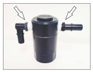
3. Assemble the quick disconnect fittings to the top of the air/oil separator as shown. Mount the straight quick disconnect on the driver side and the 90 degree on the passenger side. It is required to use Teflon tape on the fittings to ensure a proper seal. **NOTE: DO NOT over-tighten fittings in top of oil separator.** Mount the canister to the bracket using the two button head screws and lock washers.
