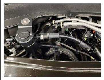
5. Install hoses on to oil separator as shown. Mount the long hose going to the PCV valve. Mount the short hose to the intake manifold. NOTE: Lightly coat the O-Ring with oil to insert easily.
