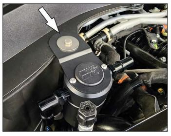
4. Mount the to the top of the cowling using M6 bolt, large flat washer and nut as shown.
