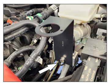
4. Install mounting bracket to brake distribution block using M8 bolt, washer and lock washer as shown.
