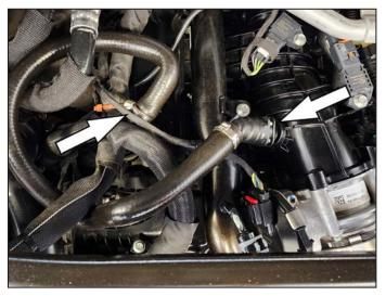
2. Remove factory PCV line by pulling tabs and removing it from the PCV valve and intake manifold
