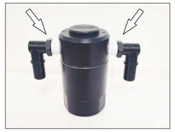
3. Assemble the quick disconnect fittings to the top of the air/oil separator as shown. It is required to use Teflon tape on the fittings to ensure a proper seal. **NOTE: DO NOT over-tighten fittings in top of oil separator.**
