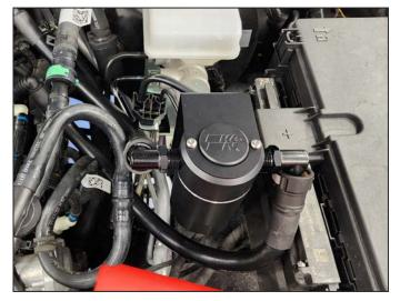
6. Install hoses on to oil separator as shown. Mount the hose with female fitting to the manifold. Mount the hose with male fitting to the PCV line going to back of the engine. **NOTE: Lightly coat the O-Ring with oil to insert easily.**
