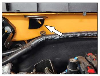
4. Remove wire harness holder on firewall and install mounting bracket using M6 nut.
