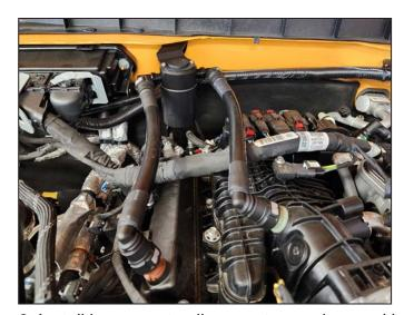
6. Install hoses on to oil separator as shown with K&N logo facing the front of the vehicle. Mount the hose on passenger side to valve cover PCV connection. Mount the hose on the driver side to the intake manifold. NOTE: Lightly coat the O-Ring with oil to insert easily.
