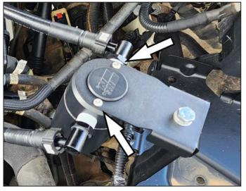
5. Mount the canister to the bracket using the two button head screws and lock washers
