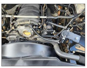
6.Looking at the K&N logo on top of the canister right-side up we can identify the inlet (dirty air from the PCV valve) install the hose from the valve cover to the inlet. The outlet (clean/filtered air going to the intake manifold) is on the right side. Route the outlet hose to the intake manifold. **NOTE: Lightly coat the O-Ring with oil to insert easily**
