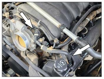
2. Remove factory PCV line by depressing grey button and removing it from the PCV valve and intake manifold
