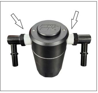
3. Assemble the quick disconnect fittings to the top of the air/oil separator. It is required to use Teflon tape on the fittings to ensure a proper seal. **NOTE: DO NOT over-tighten fittings in top of oil separator**
