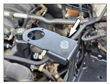
4. Mount the bracket on auxiliary battery tray mount using supplied M8 nut, lock washer and flat washer (shown in Figure)
