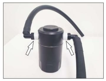
3. Assemble the quick disconnect fittings to the top of the air/oil separator as shown. It is required to use Teflon tape on the fittings to ensure a proper seal. **NOTE: DO NOT over-tighten fittings in top of oil separator.**
