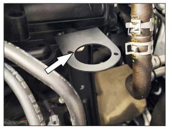
4. Install mounting bracket intake manifold by using existing M8 bolt, as shown.
