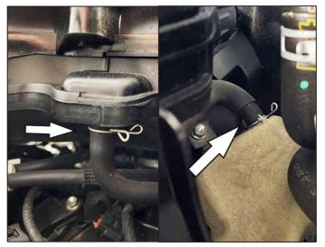
2. Remove factory PCV line at the manifold and rear of the engine by pinching clamp and moving away from end of the tubing.
