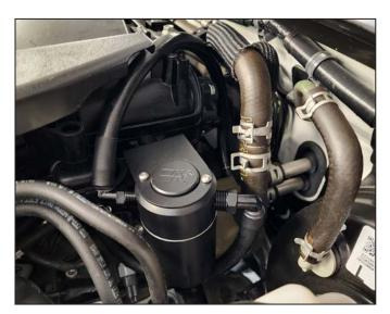
5. Mount the canister to the bracket using the two button head screws and lock washers. Mount the hose on passenger side to the rear of the engine using the stock hose clamp. Mount the hose on driver side to the intake manifold using the stock hose clamp.
