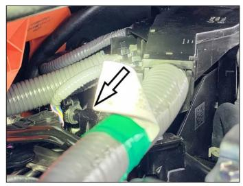
6. Insert the inlet hose to the PCV and secure using the supplied hose clamp. Then insert the outlet hose to the factory side of the hose that was removed and secure using original pinch clamp
