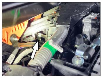
3. Remove factory PCV line that is located at the rear of the engine facing the firewall by pinching clamp and moving away from end of the tubing
