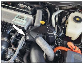
5. Install mounting bracket and canister by using existing M6 bolt and supplied button head screws and lock washers on top of the wire harness on the driver's side as shown. Route the hoses along the backside of the engine in between the firewall
