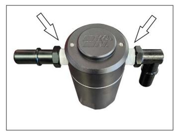
5. Assemble the quick disconnect fittings to the top of the air/oil separator as shown. It is required to use Teflon tape on the fittings to ensure a proper seal. **NOTE: DO NOT over-tighten fittings in top of oil separator**
