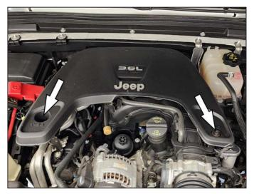
2. Remove engine cover by removing the two 10mm bolts
