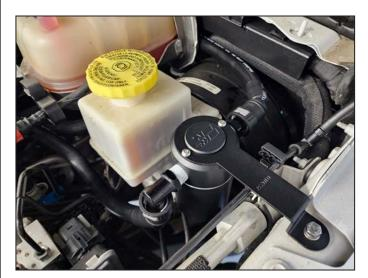
8. Install the bracket using the supplied 10mm bolt, lock washer and flat washer in the empty threaded hole on the fender shown. Mount the long hose from the valve cover to the straight fitting of the canister. Mount the short hose from the intake manifold to the 90 degree connection on the canister. **NOTE: Lightly coat the O-Ring with oil to insert easily**
