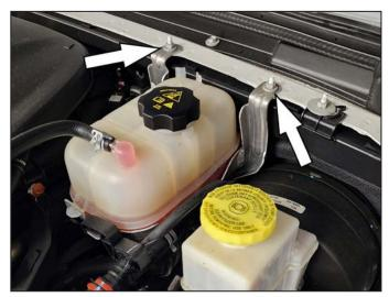
4. Remove nuts from coolant reservoir and pull up and off studs for additional clearance routing the hoses
