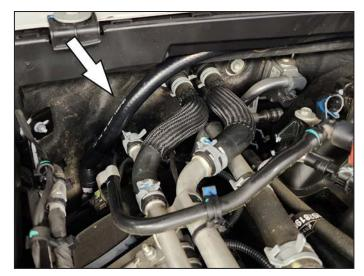
6. Route the long hose along the back of the firewall behind the coolant reservoir. Connect to the valve cover and remount the coolant reservoir
