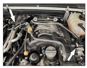
3. Remove factory PCV line by depressing the button and removing it from the PCV valve and intake manifold
