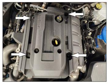
2. Remove engine cover by removing 4 bolts
