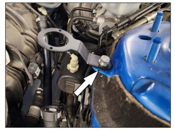
7. Install mounting bracket to strut tower tab block using M8 bolt, washer and lock washer as shown
