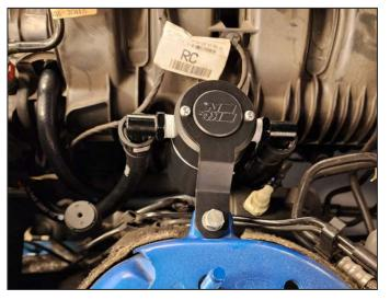
8. Mount the canister to the bracket using the two button head screws and lock washers. Ensure the K&N logo is facing as shown
