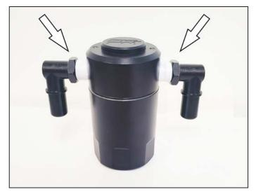
6.Assemble the quick disconnect fittings to the top of the air/oil separator. It is required to use Teflon tape on the fittings to ensure a proper seal. NOTE: DO NOT over-tighten fittings in top of oil separator
