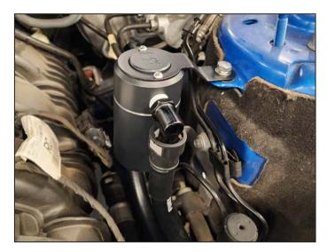
9. Install hoses on to oil separator as shown. Mount the hose with male fitting to the oil separator connector facing the rear. Mount the hose with female fitting to oil separator connector facing the front. NOTE: Lightly coat the O-Ring with oil to insert easily.
