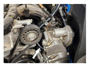
5. Connect the female 90\* connector to the intake manifold. Route the hose underneath the throttlebody towards the driver's side strut tower
