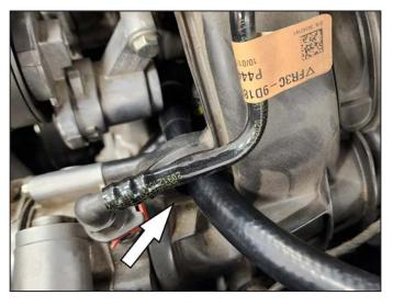
4. Install hose with male connector into OEM connector. Go through the hole in the intake manifold as shown
