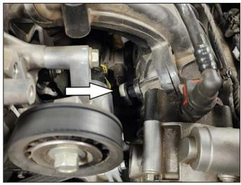
3. Remove factory PCV line by pushing button and removing it from the intake manifold. Rotate the connector slight upward
