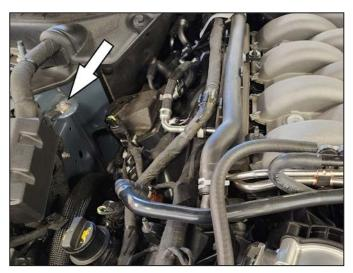
4. Remove bolt from ground-strap on the passenger side strut tower
