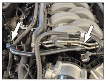
3. Remove factory PCV line by pulling tabs and removing it from the PCV valve and intake manifold
