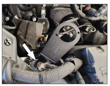
6. Mount the bracket using bolt removed from the ground-strap. Ensure the bracket is underneath the ground-strap
