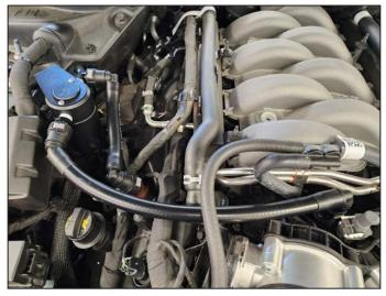
7. Install hoses on to oil separator as shown. Mount the short hose to PCV valve on the valve cover to the 90 degree fitting of the canister. Mount the long hose from the straight connection on the canister going to the intake manifold. **NOTE: Lightly coat the O-Ring with oil to insert easily**
