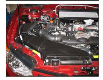
Stock air box system installed
