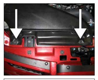
c. Remove the two mounting bolts securing the air inlet scoop and remove the scoop from the vehicle.
