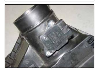
k. Remove the MAF sensor from the factory air filter housing.
