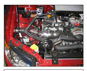
AEM® intake system installed
