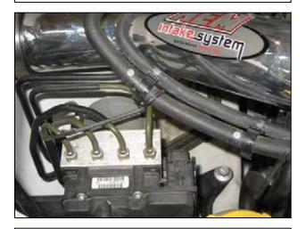
I. Secure the two rubber hoses to the steel brake tube using the supplied 6" zip-tie. Trim excess plastic.
