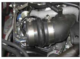
b. Install the hump hose coupler onto the stock turbo inlet tube and secure using a #44 hose clamp.
