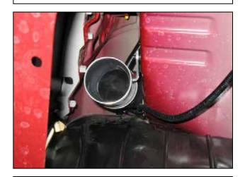
g. Install the lower intake pipe with the shorter side going into the 90° coupler. Rotate the pipe until the mounting bracket is aligned with the stud in the frame rail. Secure the intake pipe using a #48 hose clamp.
