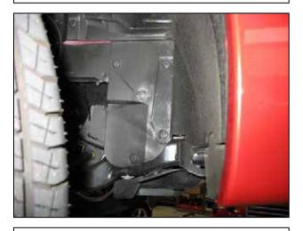
g. With the front wheels turned all the way to the right, locate the plastic clips just forward of the suspension holding the liner to the passenger side wheel well and remove them.
