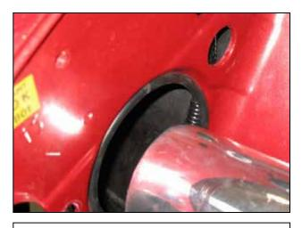
e. Install the rubber edge trim around the hole in the inner fender where the factory intake system was routed.
