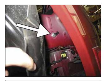
j. Locate the threaded stud behind the area where the lower resonator was mounted. Remove the nut on the stud and set it aside as it will be reinstalled later.
