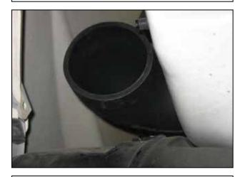
f. Install the 90° coupler by routing it through the inner fender hole and sliding it over the end of the upper intake pipe. Secure the coupler using a #44 hose clamp.
