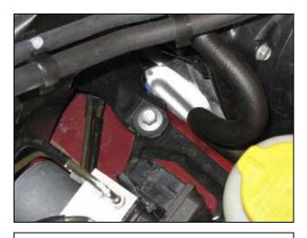
e. Down on the frame rail, on each side of the air box are the bolts that secure the air box in place. Remove the two bolts and gently lift out the air box assembly.
