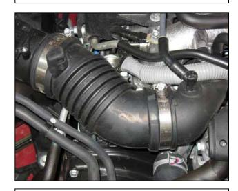
d. Loosen the two hose clamps on the stock air inlet tube and remove it.
