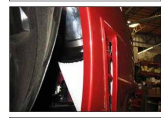
i. Install the air filter onto the end of the lower intake pipe. Push the air filter over the pipe until the stop in the air filter is reached. Use a #52 clamp to secure the air filter onto the intake pipe.
