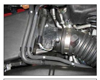
b. Unplug the mass air flow sensor (MAF) wiring harness.
