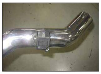
c. Using the two supplied 8-32 bolts, install the MAF sensor into the upper intake pipe.
