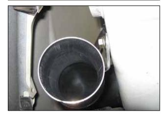
h. Install the previously removed factory M8 nut to secure the lower intake pipe. Align the lower pipe until the 90° coupler is centered in the inner fender hole and fully tighten the nut at this time.
