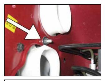
i. From the engine bay, remove the remaining nut securing the lower resonator.
