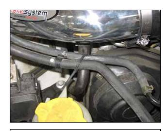
k. Secure the two rubber hoses to the rubber AC hose using the supplied 6" zip-tie. Trim excess plastic.
